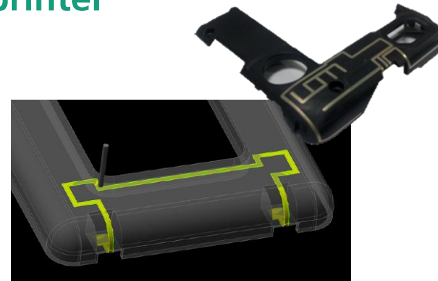
Internal electric circuit [NEOTECH]
